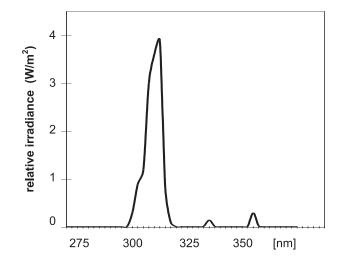
Fig. 1. Light spectrum used for ultraviolet-B irradiance.
